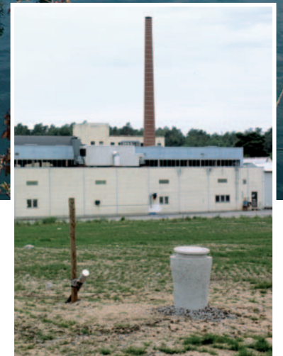
Developments down among the paper fibres can be studied through a well and through a number of pipes in the landfill site. Items for measurement include gaseous emissions and subsidence.
